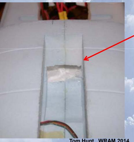
**DYNAM ME-262** Hole in aft wall of nose gear well allows air to pass over ESC's.
