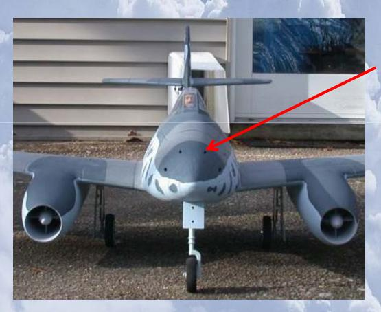
Gun ports let air into fuselage just in front of battery In DYNAM ME-262 (note: this is not a stock feature in this model!)
